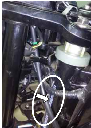
Chassis Number Location On Side of Steering Tube (Alpha-Numeric - 17 Digits)
