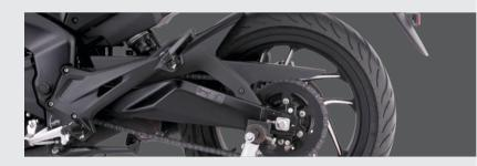
Ensure application of 9 to 11 Kgf.m torque to rear axle nut.
