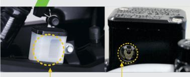
Rear Brake Fluid Reservoir Front Brake Fluid Reservoir
