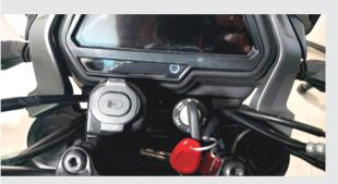
Mobile charging socket is provided near Ignition switch as an OE fitment.
