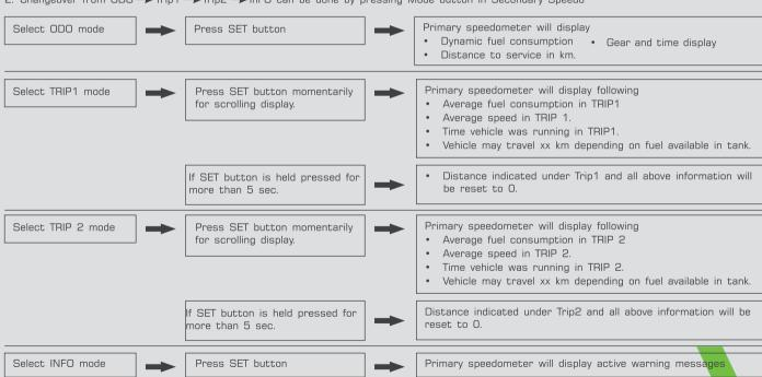
User can select any of the above screens and the screen at ignition OFF condition will be retained in next ignition ON cycle.
